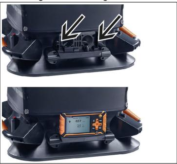
1. Make sure that the testo 420 is fully pushed into the instrument holder. In doing so, pay attention to the catch on the right-hand and left-hand side in the bracket.
