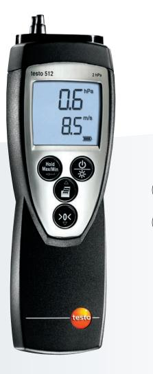
The differential pressure measuring instrument testo 512 is available in four different versions:
