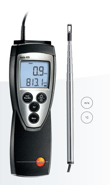
testo 425 is a compact anamometer with a fixed thermal flow velocity probe. The probe head has a diameter of 7.5 mm. With the extendable telescope (length max. 820 mm), the measuring instrument is suitable for flow velocity measurement in ducts. The testo 425 also measures extremely accurately in the low flow velocity range. The volume flow is directly shown in the display. For the purposes of volume flow calculation, the duct area can be
