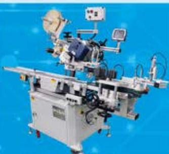
Solo Flexcy Tamp Labelling c/w TTO Printer
