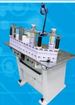
Solo Wrap-Around Body & Neck Labelling
