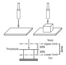
Adjusts the zone with  $\pm 10\%$  according to the light received.
