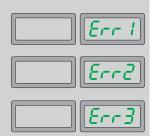
Difference of sensing level between two points is too small
