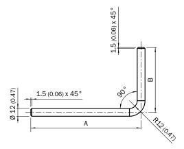
① BEF-MS12L-(N)A: A = 200 mm, B = 150 mm ② BEF-MS12L-(N)B: A = 250 mm, B = 250 mm
