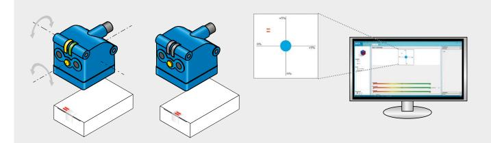
Once assembled, Glare is remarkably simple to align and commission. In "Align" mode, two LEDs attached to the sensor each cover one tilt direction (horizontal or vertical) and flash until the sensor is correctly aligned in the respective direction. The SOPAS configuration software also displays cross hairs to aid the customer in alignment and features a detailed context menu to help with installation and commissioning.
