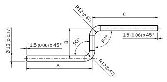
① BEF-MS12Z-(N)A: A = 150 mm, B = 70 mm, C = 150 mm ② BEF-MS12Z-(N)B: A = 150 mm, B = 70 mm, C = 250 mm BEF-RMC-D12
