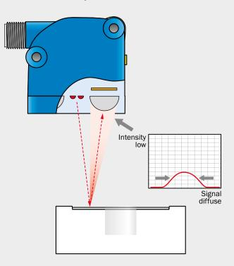
At a defined angle, visible red light lands on the object to be detected. Depending on the gloss level of the surface, the light beam is thrown back with a different intensity and scatter. This information is recorded and analyzed via two high-resolution line sensors with the patented Delta-S-Technology.
