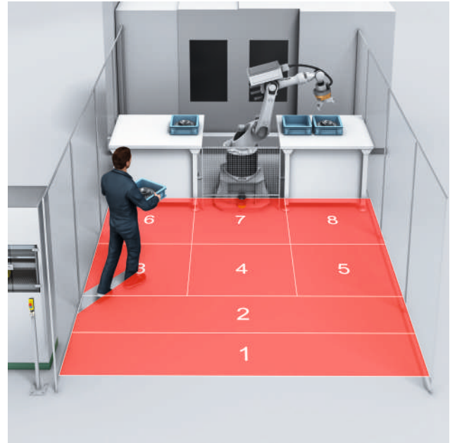
Figure 47: Simultaneous monitoring of multiple protective fields
