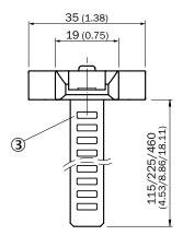
① Sensoradapter with T-slot Fixing screw ③ Strap
