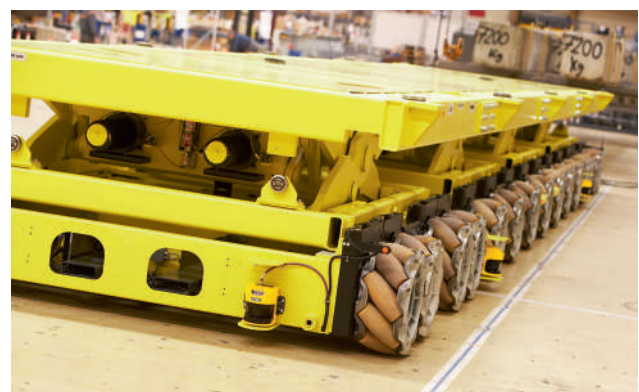
Figure 80: Hazardous area protection on an autonomous vehicle with safety laser scanners
