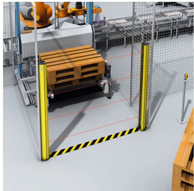
Figure 44: Access protection using a safety multibeam sensor
