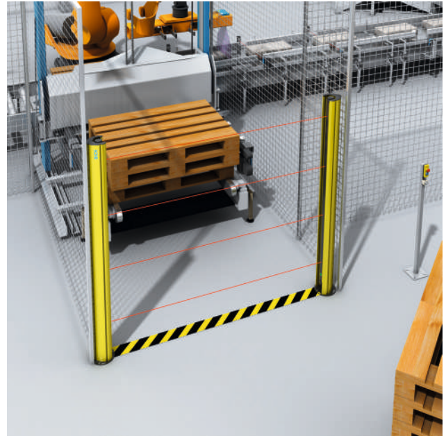
Figure 22: Initiating a stop by a safety multibeam sensor on a pallet handling machine when a person approaches
