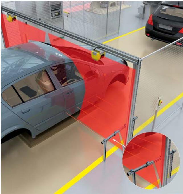
Fig. 4.2.1 Protective field switching with two safety laser scanners and four sensors arranged in parallel with time monitoring.
