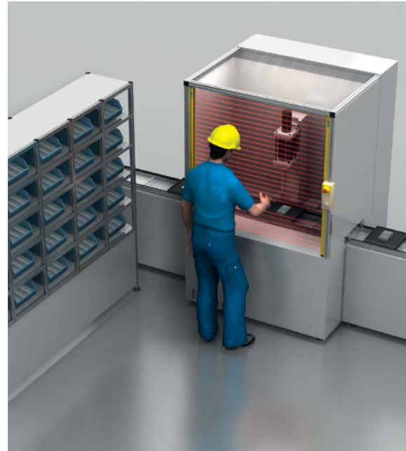
Fig. 1.3 Small opening size for physical guard.
