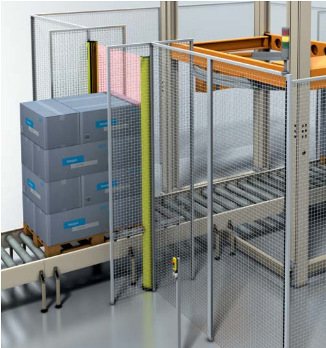
Fig. 4.1.1 Protective field muting with four sensors arranged in parallel and time monitoring
