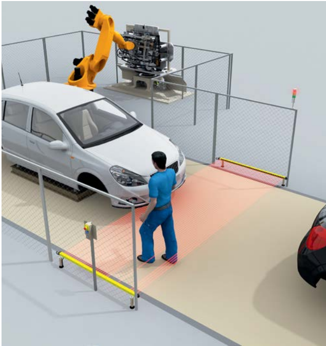
Fig. 5.1 Differentiation between humans and materials on a bodyparts carrier.
