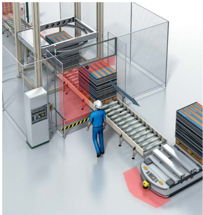
Fig. 4.2.4 Protective field switching with one safety laser scanner and four sensors arranged in parallel with time monitoring
