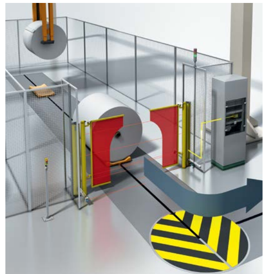
Fig. 4.1.3 Protective field muting with four sensors arranged opposite one another and additional signal
