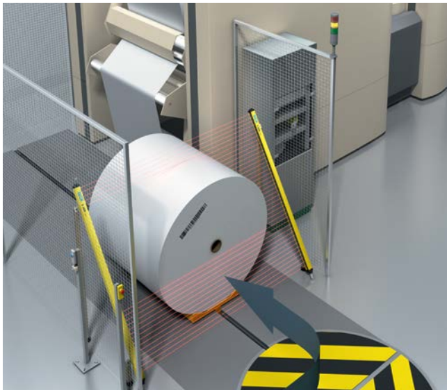
Note: In the blanked area, the detection capability of the safety light curtain, and thus the minimum distance, is enlarged (deteriorates). What is known as the effective resolution takes the blanked beams (and thus the size of the blanked area during material handling) into account.
