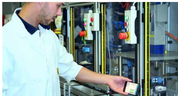
Figure 7: Safeguarding of a machine and diagnostics on the protective device
