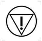
Figure 75: Symbol IEC 60417-5638: Emergency stop
