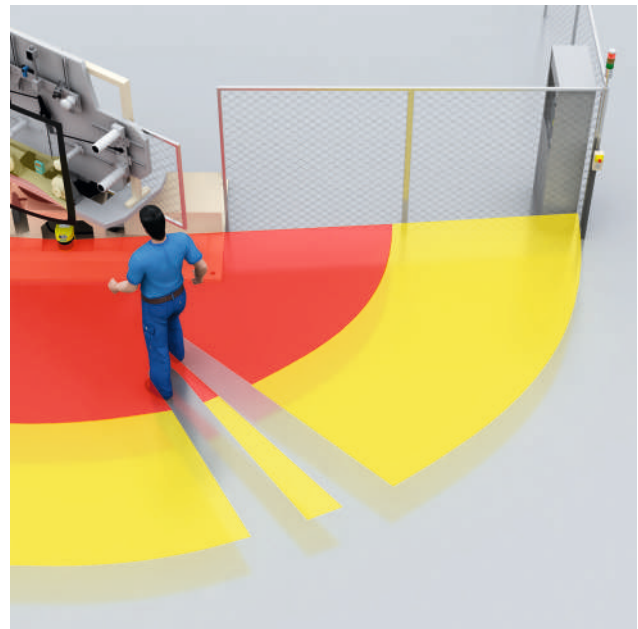
Figure 25: Initiating a stop and preventing start using a safety laser scanner (hazardous area monitoring)
