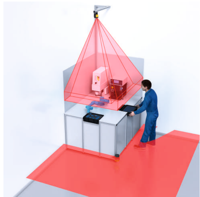
Figure 48: Protecting people when leaning into the hazardous area of a collaborative robot using a 3D vision-based camera system
