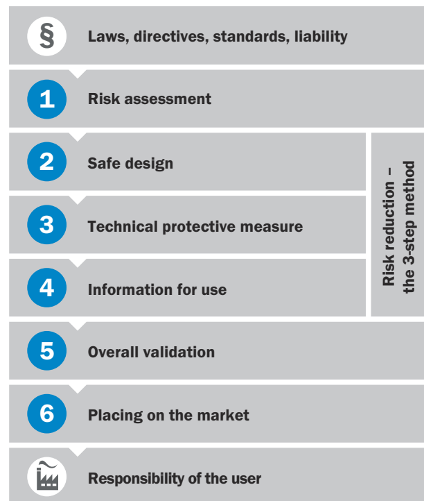
Figure 2: Structure: “Six steps to a safe machine”
