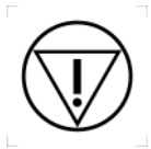
Figure 75: Symbol IEC 60417-5638: Emergency stop
