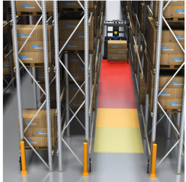
Figure 30: Adapting the monitored area of a safety laser scanner according to the vehicle speed
