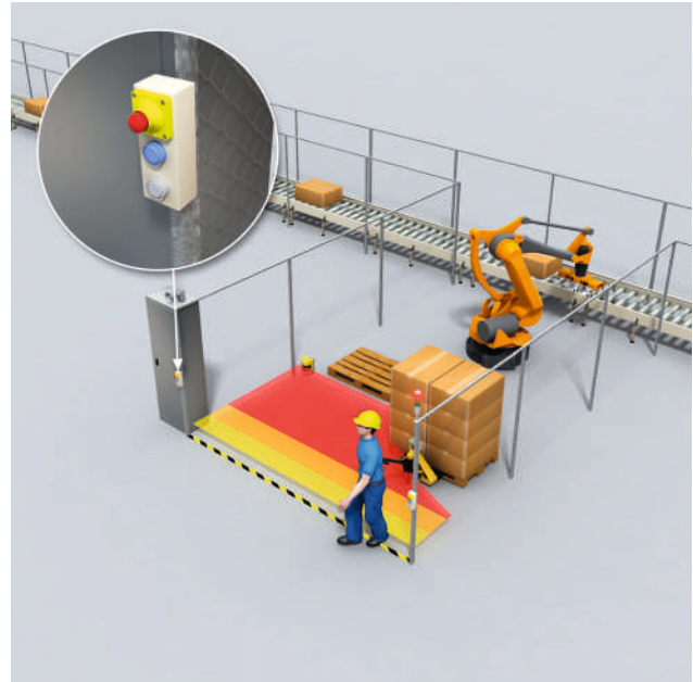
Figure 72: Emergency stop and reset control switches at a robot station
