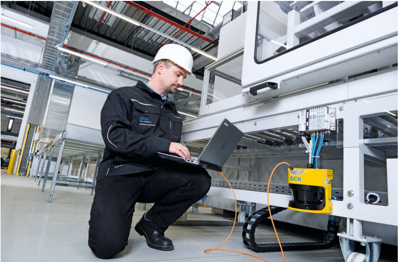
Figure 125: Service employee from SICK performing an overall validation of a machine
