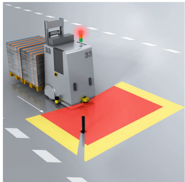
Figure 82: Positioning of a test body on an autonomous vehicle for testing the detection of a standing person
