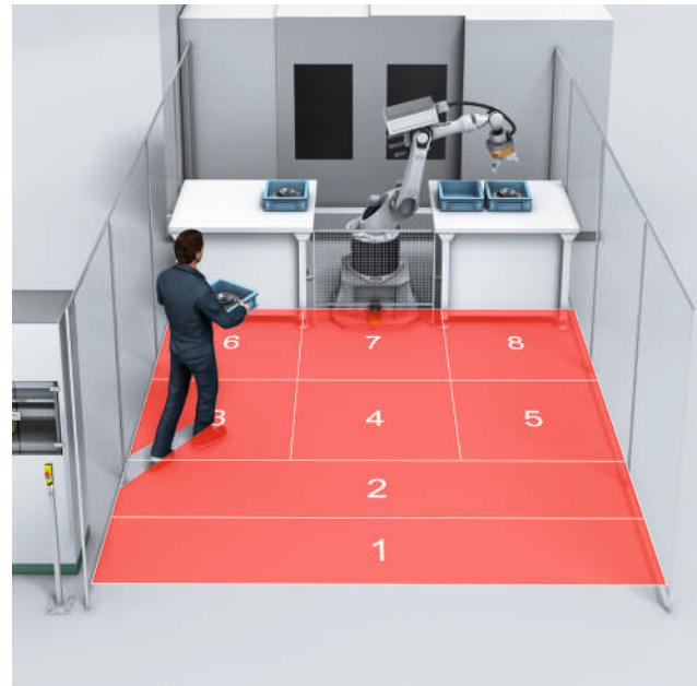
Figure 47: Simultaneous monitoring of multiple protective fields
