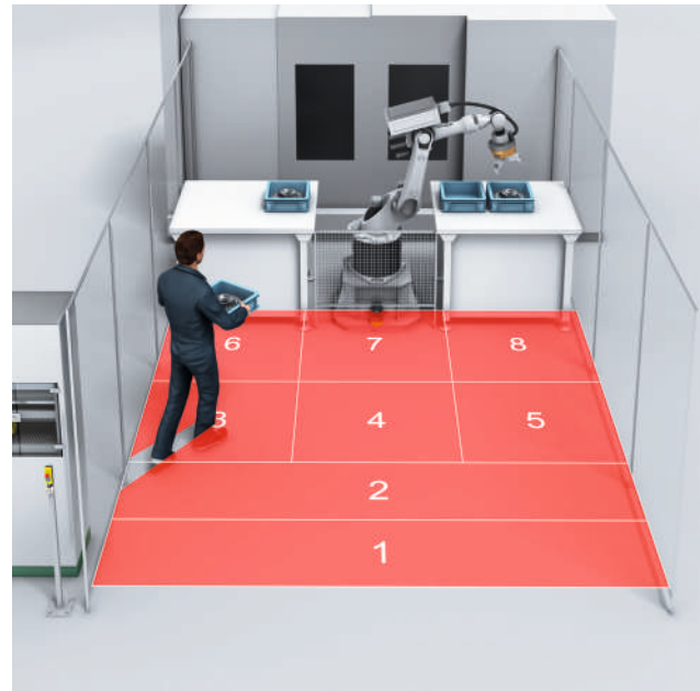
Figure 47: Simultaneous monitoring of multiple protective fields
