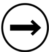
Figure 4: Symbol for positive-opening normally closed contacts in accordance with EN 60947-5-1, Annex K
