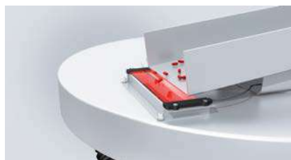
Detection of free falling tablets
