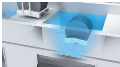
Wafer detection in wet process
