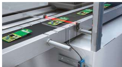
Leading edge detection for PCBs
