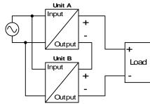
Pay attention that leakage current, EMI, inrush current, harmonics will increase when using multiple devices.
