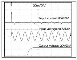
Fig. 5-2 Input inrush current, zoom into first peak 230Vac input, 24V 5A output, 40°C ambient
