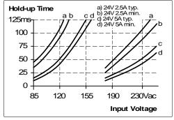
Fig. 7-2 Shut-down behaviour, definitions
