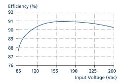
Fig. 8-3: Efficiency vs. input voltage at 24V, 1.5A, typ.
