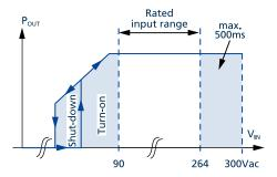
Fig. 3-1: Input voltage range
