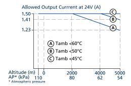
Fig. 15-2: Output power vs. altitude
