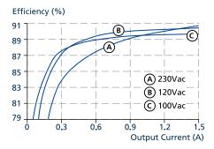
Fig. 8-1: Efficiency vs. output current at 24V, typ.
