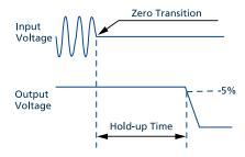
Fig. 7-2: Shut-down behaviour, definitions
