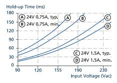
Fig. 7-1: Hold-up time vs. input voltage
