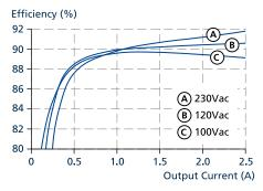
Fig. 8-1: Efficiency vs. output current at 24V, typ.
