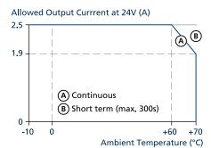
Fig. 15-1: Output power vs. ambient temp.
