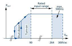
Fig. 3-1: Input voltage range
