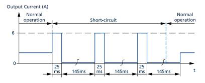
Fig. 6-2: Intermittend current at short circuit, typ.\*)
