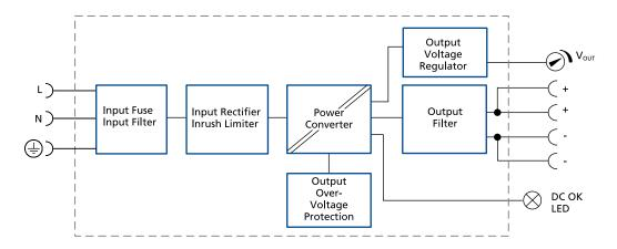
Fig. 11-1: Functional diagram
