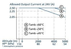
Fig. 15-2: Output power vs. altitude
