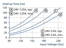
Fig. 7-1: Hold-up time vs. input voltage
