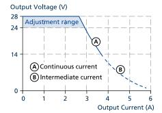
Fig. 6-1: Output voltage vs. output current, typ.
