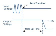
Fig. 7-2: Shut-down behaviour, definitions
