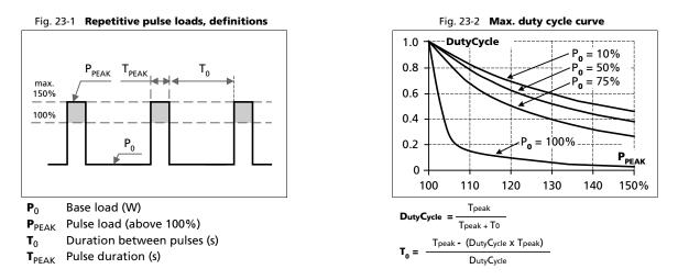
**Example:** A load is powered continuously with 60W (= 50% of the rated output load). From time to time a peak power of 180W (= 150% of the rated output load) is needed for 1 second.
