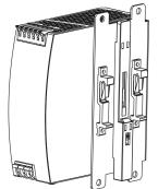
Side mounting with DIN rail brackets
