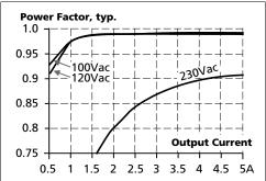
Aug. 2021 / Rev. 2.5 DS-QS5.241-EN All parameters are specified at 24V, 5A, 230Vac, 25°C ambient and after a 5 minutes run-in time unless otherwise noted.
