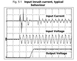
Aug. 2021 / Rev. 2.5 DS-QS5.241-EN All parameters are specified at 24V, 5A, 230Vac, 25°C ambient and after a 5 minutes run-in time unless otherwise noted.
