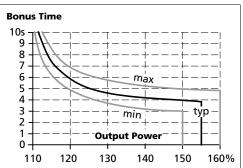
The BonusPower® is available as soon as power comes on and immediately after the end of an output short circuit or output overload.
