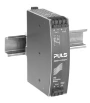
as decoupling devices included. It can be used for various purposes. The most popular application is to configure highly reliable and true redundant power supply systems. Another interesting application is the separation of sensitive loads from non-sensitive loads. This avoids the distortion of the power quality for the sensitive loads which can cause controller failures.
