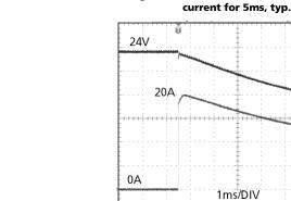
Peak load 10A (resistive) for 50ms Output voltage dips from 24V to 20V. Voltage
