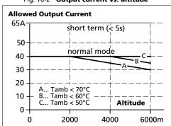
Fig. 10-2 Output current vs. altitude
