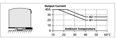
Fig. 26-9 Mounting Orientation D (Horizontal cw)
