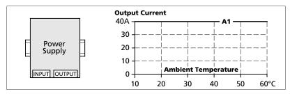
Fig. 26-7 Mounting Orientation B (Upside down)
