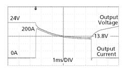
200A Peak load (resistive) for 5ms Output voltage dips from 24V to 13.8V.
