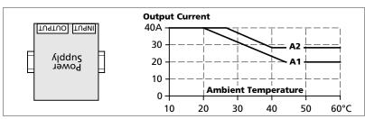
Fig. 26-8 Mounting Orientation C (Table-top mounting)
