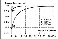
Dez. 2020 / Rev. 1.3 DS-QS40.241-EN All parameters are specified at 24V, 40A, 230Vac, 25°C ambient and after a 5 minutes run-in time unless otherwise noted.
