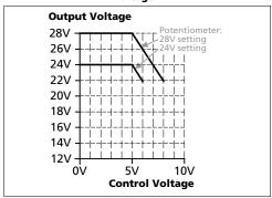
Fig. 10-2 Applying the control voltage
