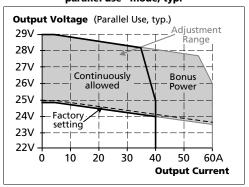
Fig. 6-4 Dynamic overcurrent capability, typ.
