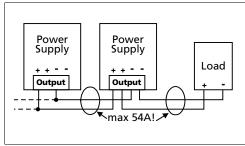
Fig. 15-2 Using distribution terminals
