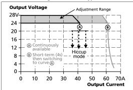
Fig. 6-3 Short-circuit on output, Hiccup<sup>PLUS</sup> mode, typ.
