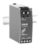
The YR80.242 is equipped with two input channels (40A each), which are individually decoupled by utilizing mosfet technology. The output current can go as high as 80A. Using mosfets instead of diodes reduces the heat generation and the voltage drop between input and output. The YR80.242 does not require an additional auxiliary voltage and is self-powered even in case of a short circuit across the output.
