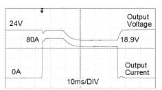
80A Peak load (resistive) for 50ms Output voltage dips from 24V to 18.9V.
