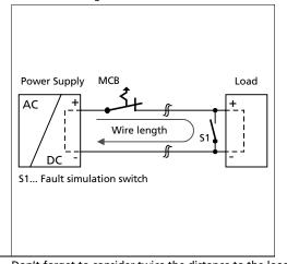
Maximal wire length\*) for a fast (magnetic) tripping:
