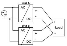
If more than three units are connected in parallel, a fuse or circuit breaker with a rating of 50A or 63A is required on each output. Alternatively, a diode or redundancy module can also be utilized.
