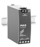
The YR40.482 is equipped with two input channels (20A each), which are individually decoupled by utilizing mosfet technology. The output current can go as high as 40A. Using mosfets instead of diodes reduces the heat generation and the voltage drop between input and output.
