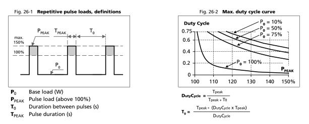
**Example:** A load is powered continuously with 480W (= 50% of the rated output load). From time to time a peak power of 1440W (= 150% of the rated output load) is needed for 1 second.
