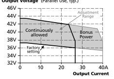
Fig. 6-4 Dynamic overcurrent capability, typ.
