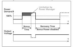
The BonusPower® is available as soon as power comes on and after the end of an output short circuit or output overload.
