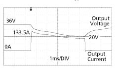
53.4A Peak load (resistive) for 50ms Output voltage dips from 36V to 28.2V. 133.5A Peak load (resistive) for 5ms Output voltage dips from 36V to 20V.
