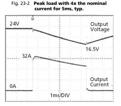
Peak load 16A (resistive) for 50ms Output voltage dips from 24V to 18.5V. Peak load 32A (resistive) for 5ms Output voltage dips from 24V to 16.5V.
