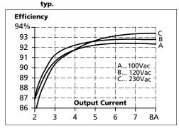
Efficiency vs. output current at 24V,
