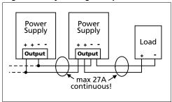
Fig. 12-2 Using distribution terminals
