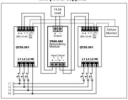
Fig. 21-7 Typical N+1 Redundant configuration for 40A with two dual redundancy modules and four power supplies
