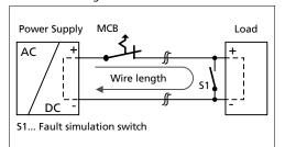
Maximal wire length\*) for a fast (magnetic) tripping:
