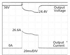
26.6A Peak load (resistive) for 50ms Output voltage dips from 36V to 24.4V.
