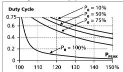
$$DutyCycle = \frac{T_{peak}}{T_{peak} + T_0}$$
