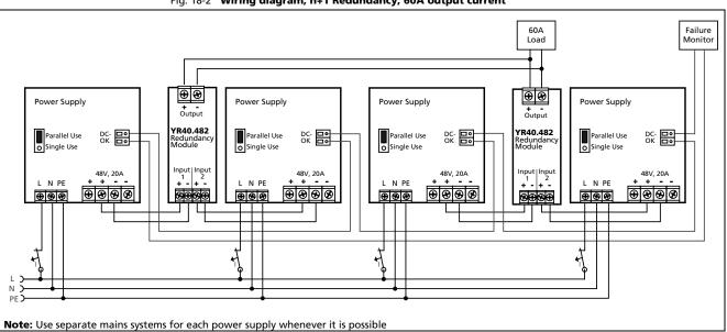
Fig. 18-2 Wiring diagram, n+1 Redundancy, 60A output current
