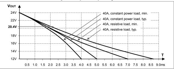
Fig. 8-2 Hold-up time vs. input voltage
