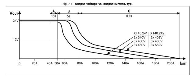
Zone **A**: 25% extra output power for typ. 15s Zone **B**: 100% higher output current for typ. 5s Zone **C**: Quick-acting shut-down after typ. 0.1s
