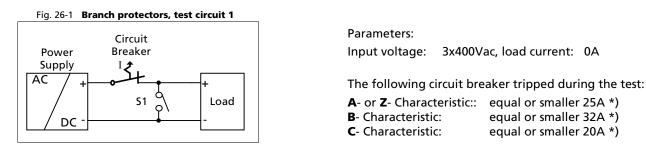
Test 2: Short circuit with S1 on the load end (additional impedance included; represents longer load wire length).
