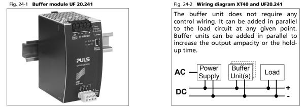
Do not use the buffer module to bridge mains interruptions which are longer than typ. 350ms. Once the mains is off for longer than typ. 350ms, the XT power supply needs an additional 1s to restart again.
