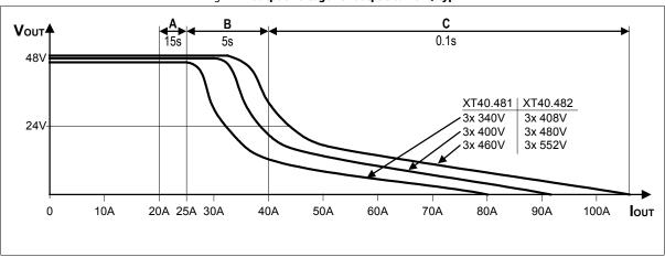
Fig. 7-1 Output voltage vs. output current, typ.
