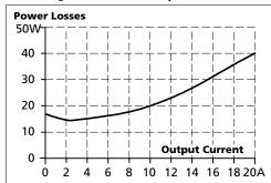
Fig. 9-4 Losses vs. input voltage, 48V, 20A
