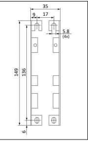
Fig. 20-6 Wall/panel mounting, side view
