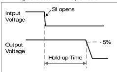
Note: At no load, the hold-up time can be up to several seconds. The green DC-ok lamp is also on during this time.
