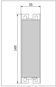
Fig. 20-5 Hole pattern for wall mounting
