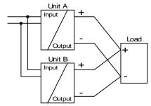
150% of the rated output current of one DC/DC-converter. Keep an installation clearance of 15mm (left / right) between two DC/DC-converters and avoid installing the DC/DC-converters on top of each other. Do not use DC/DC-converters in parallel in mounting orientations other than the standard mounting orientation (input terminals on the bottom and output terminals on top of the unit).
