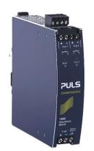
The YRM2.DIODE is a dual redundancy module, which can be used to build 1+1 and N+1 redundant systems. It is equipped with two input channels, which are individually decoupled by utilizing diodes.
