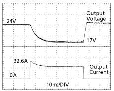
32.6A Peak load (resistive) for 50ms Output voltage dips from 24.5V to 17V.
