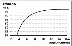
Fig. 9-2 Losses vs. output current, typ.
