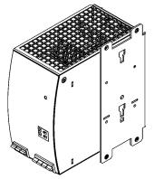
Side mounting without DIN-rail brackets
