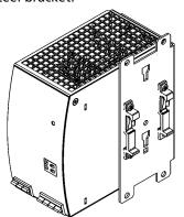
Side mounting with DIN-rail brackets
