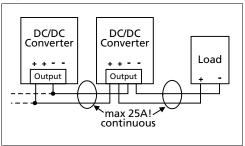
Fig. 12-2 Using distribution terminals
