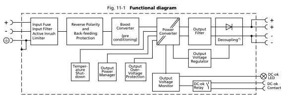
\*) Decoupling: This feature utilizes a Mosfet instead of a diode in order to minimize the voltage drop and power losses.
