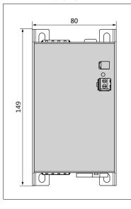
Fig. 22-5 **Hole pattern for wall mounting**
