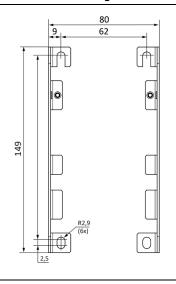
Fig. 22-6 Wall/panel mounting, side view
