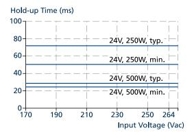
Fig. 7-1: Hold-up time vs. input voltage
