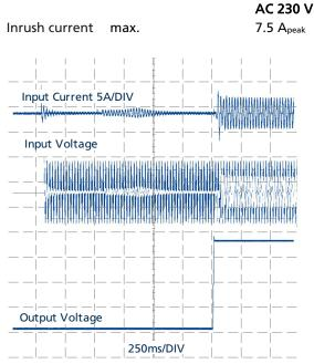
Fig. 5-1: Typical turn-on behavior at nominal load and 25 °C ambient temperature
