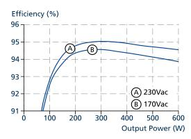
Fig. 9-1: Efficiency vs. output power at 24 V, typ.
