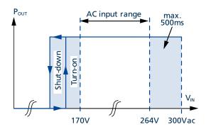
Fig. 3-1: Input voltage range
