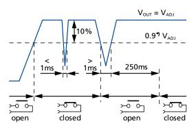
Fig. 8-1: Output-OK relay contact behavior
