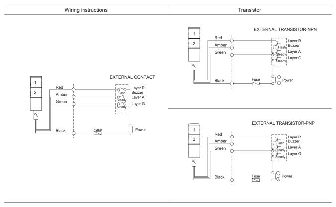
• External power line/ external signal line - UL1015 AWG18(0.75sq) x 4C 400mm
