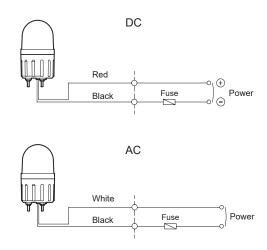
• External power line - UL1015 AWG18(0.75sq) x 2C 400mm
