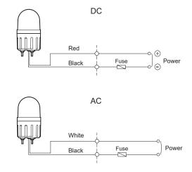
• External power line - UL1015 AWG18(0.75sq) x 2C 400mm
