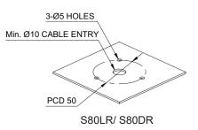
• Please refer to the dimensions below for installation of mounting brackets
