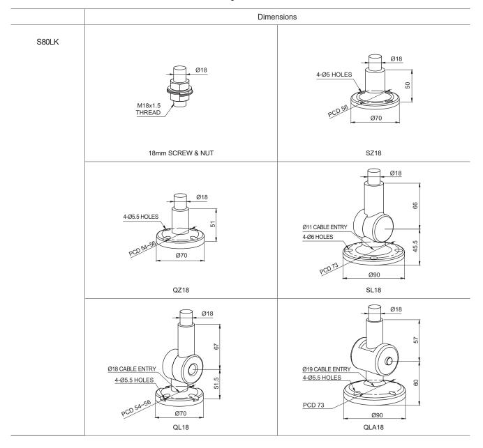
· Please refer to the dimensions below for installation of mounting brackets
