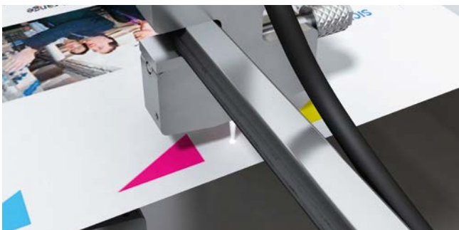
Detecting registration marks on printing machines.
