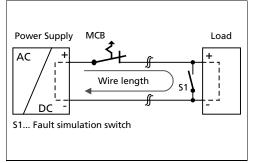
Maximal wire length\*) for a fast (magnetic) tripping:
