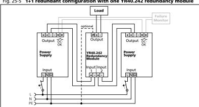
Fig. 25-5 1+1 redundant configuration with one YR40.242 redundancy module
