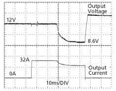
Fig. 25-3 **48A peak current for 12ms , typ. (3x the nominal current)**
