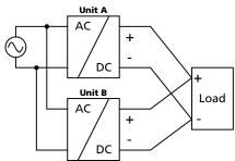
If more than three units are connected in parallel, a fuse or circuit breaker with a rating of 25A or 32A is required on each output. Alternatively, a diode or redundancy module can also be utilized.
