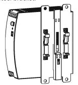
Side mounting with DIN rail brackets
