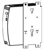
Side mounting without DIN rail brackets
