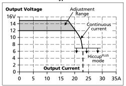
Fig. 6-2 **Dynamic output current capability, typ.**
