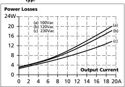
Fig. 10-4 Losses vs. input voltage at 12V, 16A, typ.
