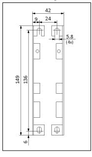
Fig. 24-6 Wall/panel mounting, side view
