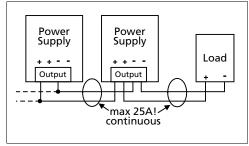
Fig. 14-2 Using distribution terminals
