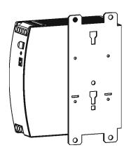
Side mounting without DIN rail brackets
