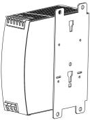
Side mounting without DIN rail brackets
