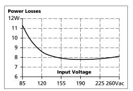
Aug. 2021 / Rev. 2.4 DS-QS5.DNET-EN All parameters are specified at 24V, 3.8A, 230Vac, 25°C ambient and after a 5 minutes run-in time unless otherwise noted.
