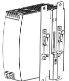
Side mounting with DIN rail brackets
