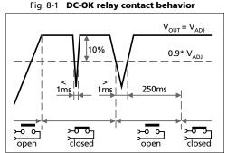
Note: The DC-OK feature requires that the output voltage reaches the nominal level after turn-on in order to function according to specification. If this level cannot be achieved, the overload LED will be on and the DC-OK contact will be open. The overload signal will only shut off as soon as the adjusted voltage is reached.
