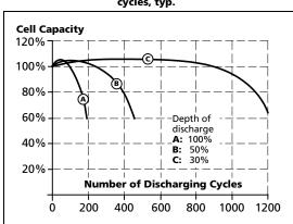
Fig. 13-2 Battery degradation vs. discharging cycles, typ.
