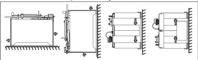
Do not use the battery module in an upside down position:
