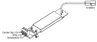
The use of the sensor board is optional, the DC-UPS will also function without the sensor board installed.
