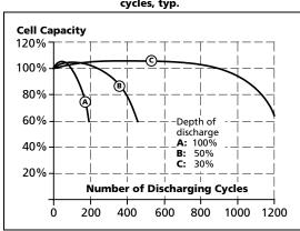
Fig. 15-2 **Battery degradation vs. discharging** cycles, typ.
