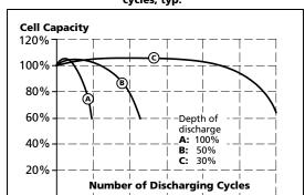
Fig. 13-2 **Battery degradation vs. discharging** cycles, typ.
