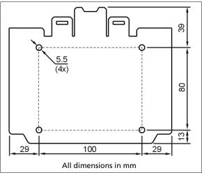
Fig. 12-3 Hole pattern for bottom mount
