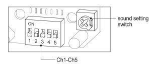
• Standard unit has 5 built-in sound tones. select different built-in sounds using the sound setting switch.
